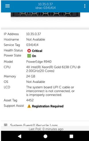
Figure 5. View—registration required—option on server dashboard
