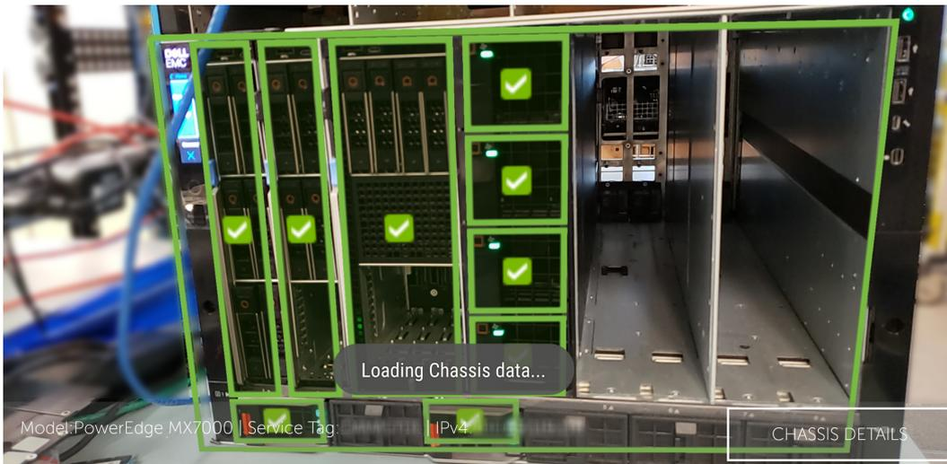
Figure 2. Monitor MX7000 chassis by using AR
